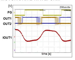
Condition: VCC = 12V, PWM input duty =100% CVCC = 10µF
